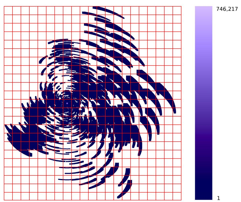
The distribution of grid updates across tiles is highly uneven, leading to poor load balance. Ordering tiles by the number of visibilities and processing from highest to lowest mitigated this. A different approach was needed on the GPU to handle the highly concentrated central region.
