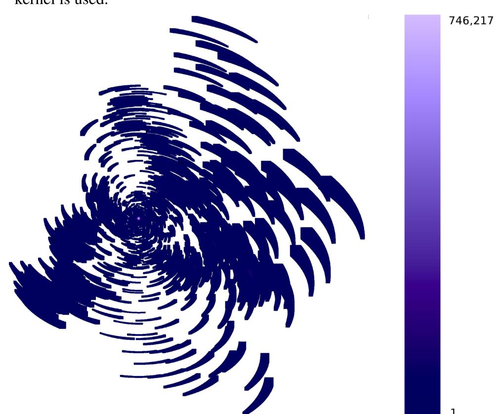
This plot shows the number of times each grid point is updated for simulated Square Kilometer Array (SKA) data. Note the extremely high concentration near the centre, a feature of this telescope. The gridding algorithm is difficult to optimize because:
