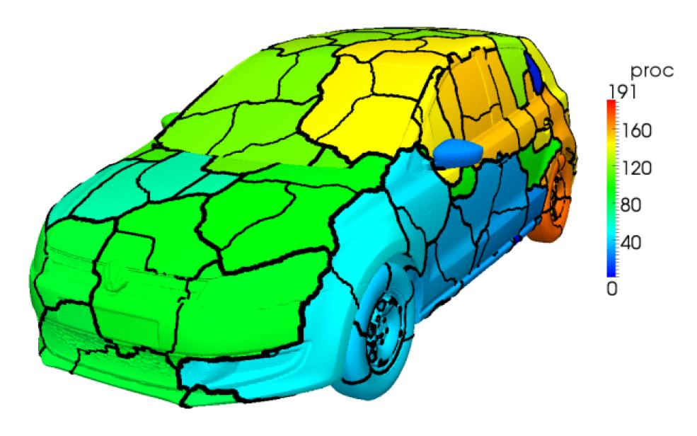
Geometry of the Polo Mk V car body with mesh decomposition over 192 cores. NAG performed external aerodynamics simulations of this real car model on the ARCHER supercomputer to validate the software deployment and perform scaling studies.
