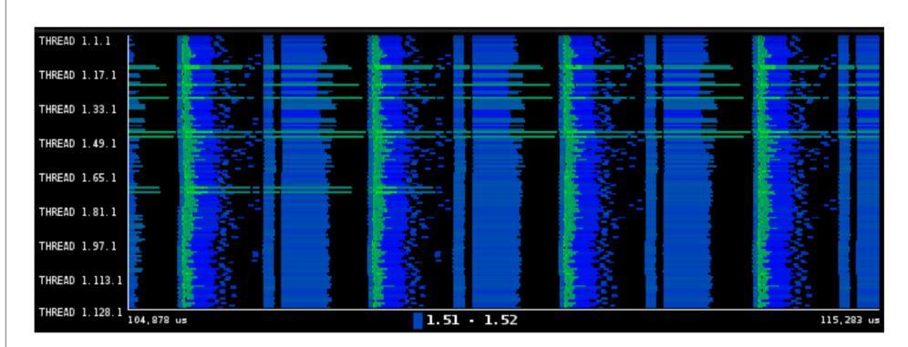
A recommendation was made was to improve the locality of data in order to reduce the cache misses. The CFD mesh used in the simulation gets decomposed into cells (domains). The new implementation now calls renumberMesh[] which renumbers the cell list during the initialization phase.
