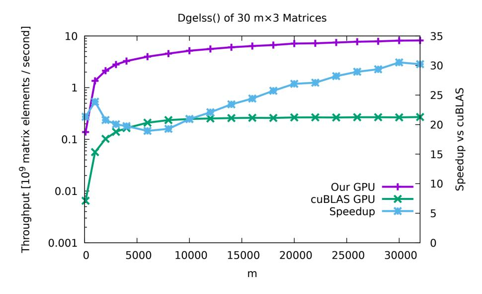
This graph shows our code vs. the NVIDIA libraries for 30 double precision m by 3 matrices. Our code is much faster. Results for different size batches and matrices and for single precision are similar.
