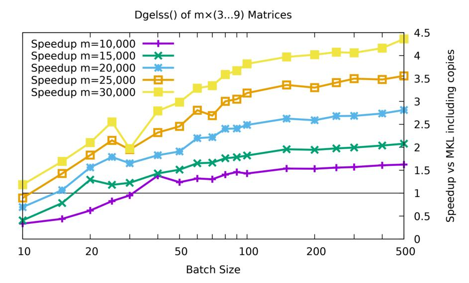
This plot shows speedup vs. MKL including transfers for batches where each matrix has m rows and a random Uniform(3, 9) number of columns.
