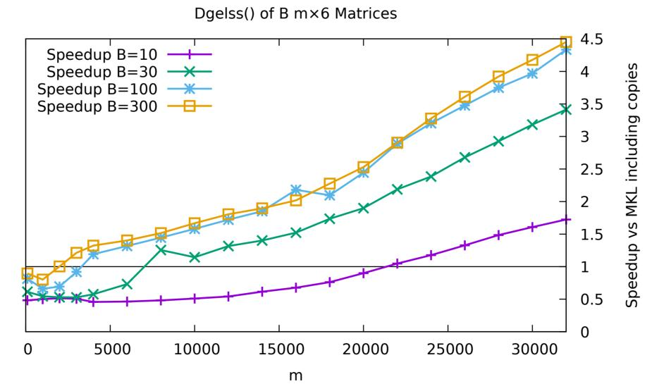
The plot above shows speedup vs. MKL including all transfers for batches of m by 6 matrices. Larger problem sizes give larger speedups.
