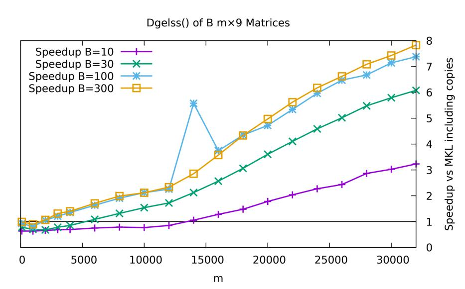
These plots show results for batches of m by 9 and m by 15 matrices. The speedups increase strongly the more columns each matrix has.
